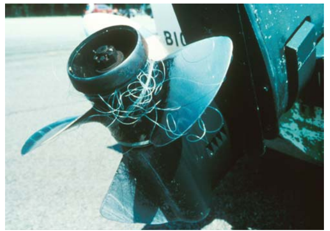
Figure 2- Discarded fishing line in boat propeller. Photo from MMRP web site.
